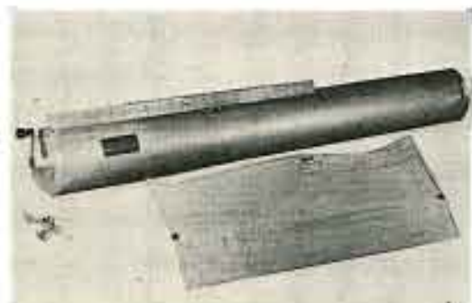
Figure 6 A 74-mc cavity resonator. The plate at left, removed from window to show inner conductor, is connected to the coupled loop and coax connector to excite the cavity.
